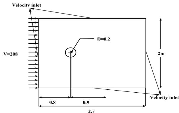
Fig. 1. Geometry of cylinder considered for simulation of unsteady vortex
