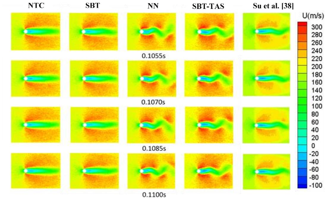
**Figure 2:** Contours of stream-wise velocity (m/s) at different times for the vortex shedding behind a cylinder using  $4 \times 10^6$  total initial number of particles and division size equal to  $200 \times 150$  cell for all NTC, SBT, NN, SBT-TAS (PPSC=3) collision schemes. The last column corresponds to Su et al. work [2] obtained using NTC-TAS.
