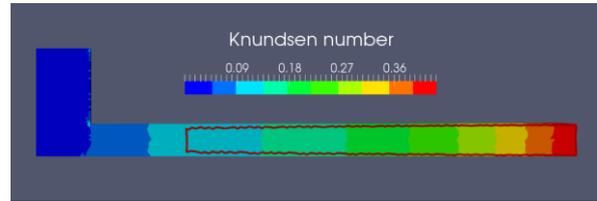
**Figure 3:** Knudsen number contour, isoline indicates  $Kn=0.1$ .
