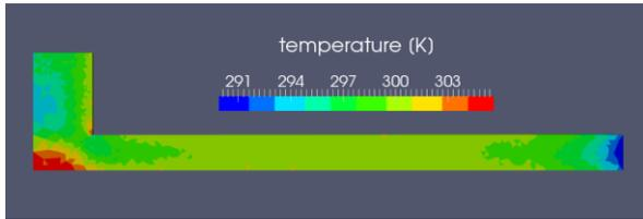
**Figure 2:** Temperature contour of flow case, Stagnation point ~305 K i.e. warmer than surface.
