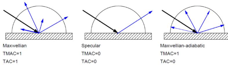
**Figure 1:** Alternative “insulated-Maxwellian” composed of three types of wall kernels.
