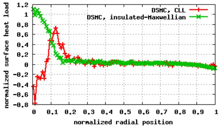
**Figure 4:** Heat load profiles on bottom surface.
